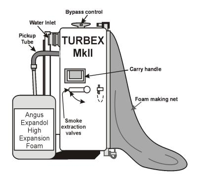
Each **HI-COMBAT** Turbex utilises forced air technology and is powered by an enclosed maintenance free water turbine driving an aerofoil fan, so that only a pressurised water supply is required for operation with Angus Expandol High Expansion Foam concentrate, consumed at typically 4.5litres/min. A special in-built filter system protects the turbine and inductor from blockage due to solid particles in the water supply.
